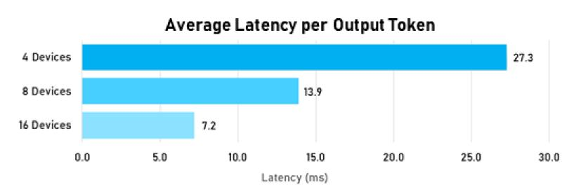
Millisecond (7.2ms) to generate an output token during GenAl inference
